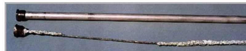
New Anode vs: Sacrificed Anode
